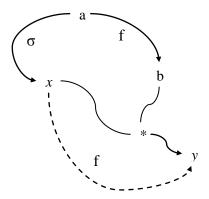
Matching is by subgraph isomorphism, i.e., we seek an isomorphism between the pattern graph and some subgraph of the data graph. Note that the rule graph contains no distinguished "variable" nodes; the only special notation needed is of the consequent edges. Use of the variable-style syntax x and y in the figure above is purely expository. All nodes matched by the rule test will have an isomorphic counterpart in the data graph, and those nodes are implicitly used in creating the resulting edges.
